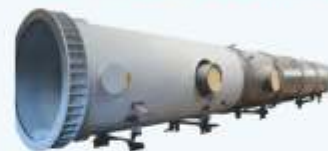
Distillation Column SS
